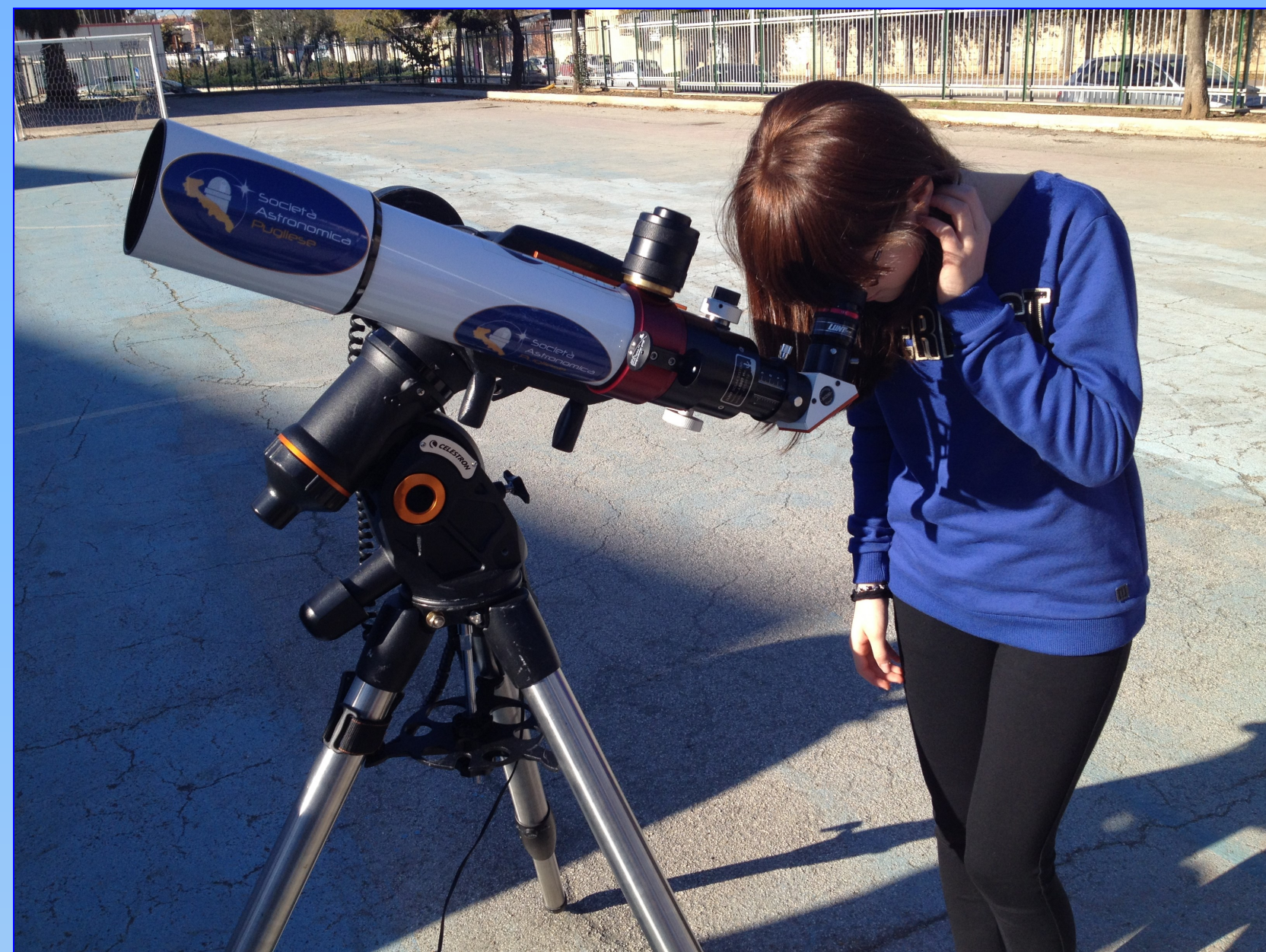
Direct observation of the sun with 80 mm Lunt Solar H-Alpha telescope.
