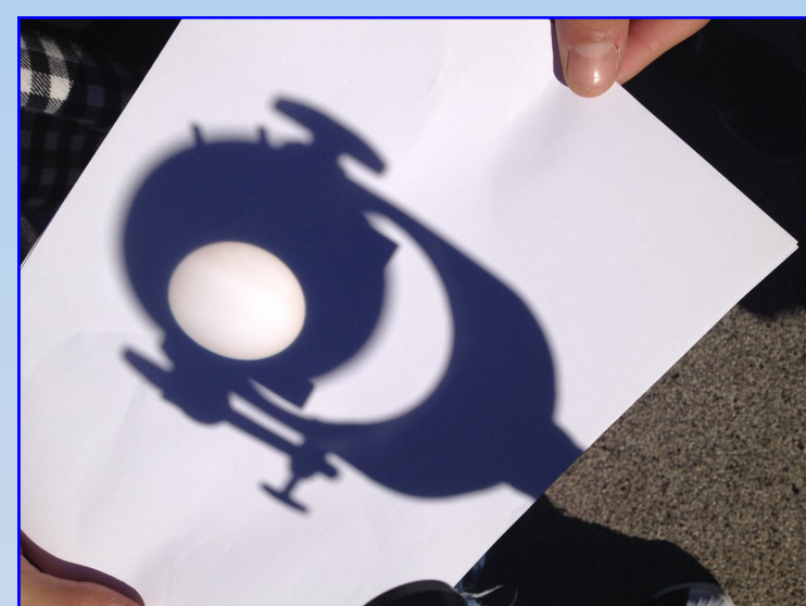
Indirect observation of the sun with telescopic projection
